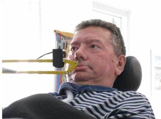
**Figure 6.8:** The webcam is mounted on the arm of an office lamp and placed close to Birger's eye.
