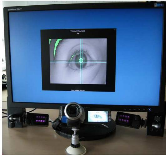
**Figure 4.3:** ITU Gaze Tracker in a remote configuration. The hardware components used are a videocamera with night vision mode and a pair of infrared light sources.
