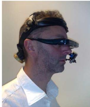
**Figure 6.10:** The user wears a head-mounted gaze tracker and interacts with the information shown on the head-mounted display.
