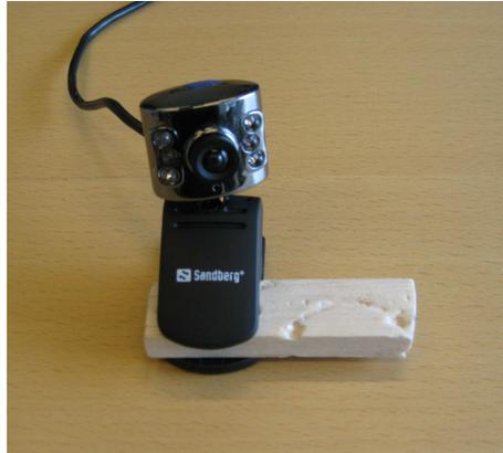
**Figure 4.2:** Webcam mounted on a piece of balsa wood that the user bites.
