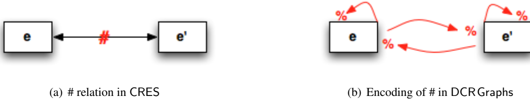
Figure 2: Encoding conflicting events in CRES as mutual excluding events in DCR Graphs
