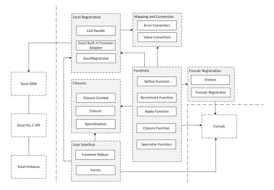
FIGURE 5.1: Overall design of Funsheet and how it integrates with Excel-DNA and Funcalc.
