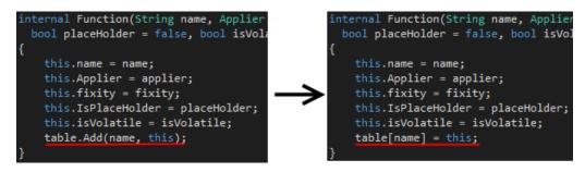
FIGURE B.2: Changes made to the constructor of the Function class.
