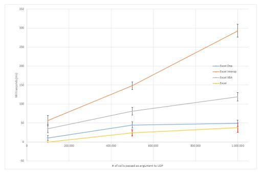
FIGURE 4.5: Average-benchmark: Excel-DNA is the best performer of the three addins. Detailed data can be found in table 4.3.
