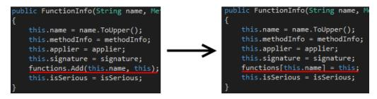
FIGURE B.3: Changes made to the constructor of the FunctionInfo class.
