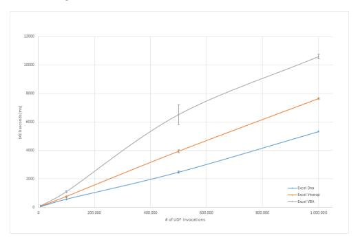
FIGURE 4.3: Random benchmark: Excel-DNA is the best performer of the three addins. Detailed data can be found in table 4.1.
