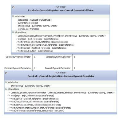
FIGURE 6.3: Design Class diagram illustrating the two visitors, the CorecalyDynamicCellVisitor and the CorecalcDynamicExprVisitor.
