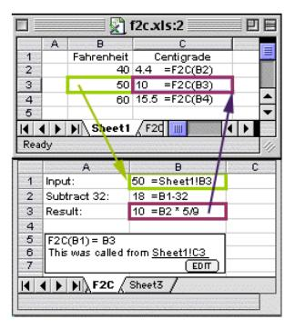
FIGURE 2.1: Invocation and definition of a SDF[2].
