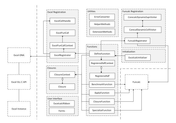
FIGURE 6.1: Class diagram of Funsheet.
