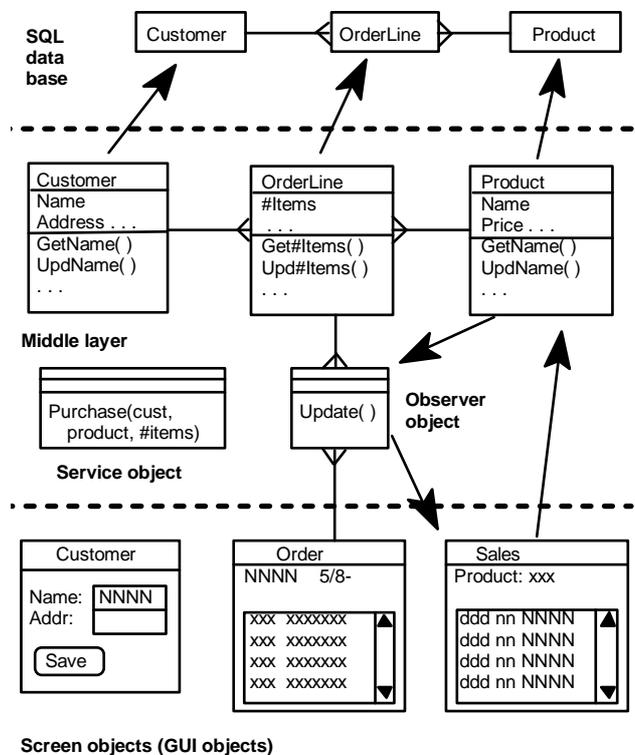
Figure 3. The complex business system architecture. The middle layer consists of degenerate objects. The database envelopes serve as buffers for screen updating. The arrows show calls between objects. Notice the two-way calls.
