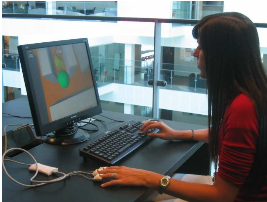
Fig. 4 The setup of the experiment. The Maze-Ball game is viewed on screen; the IOM bio-sensing hardware is placed on the subject's left hand in this picture.
