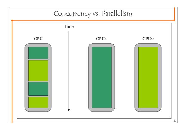
Two programs cannot execute simultaneously using one CPU. But we can create the illusion of parallelism by using multiple threads and assigning them slices of CPU time to run in.
