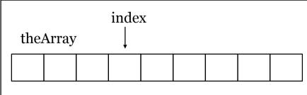
if index<theArray.length then index refers to the head of the iterator. else the iterator is empty
