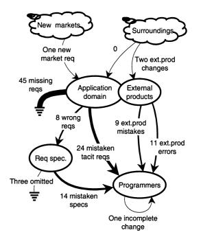
Fig. 2. How requirements pass to programmers or get lost. Arrow thickness and numbers indicate requirements 'lost' on the way. (Based on an analysis of 107 requirement defect reports.)
